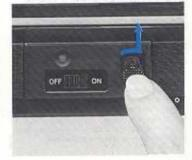
Fold out the rewind crank and turn it in the direction indicated by the arrow on it until the red Safe Load Signal bar moves out of the window to the left. You will then feel tension on the film increase and disappear, and the crank will turn freely.
