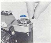
4. When you are certain that the film is completely rewound, pull the back-cover release knob to open the back and remove the cartridge.
