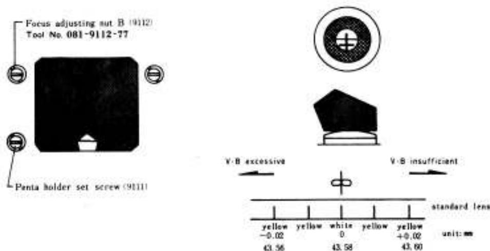
3. After the adjustment, operate the mirror several times, rotate of the standard lens, and make sure that, when vertical lines of the chart image coincide, the standard values ( $43.58 \pm 0.02\text{mm}$ ) are not exceeded and that no "half fuzziness" is observed.
