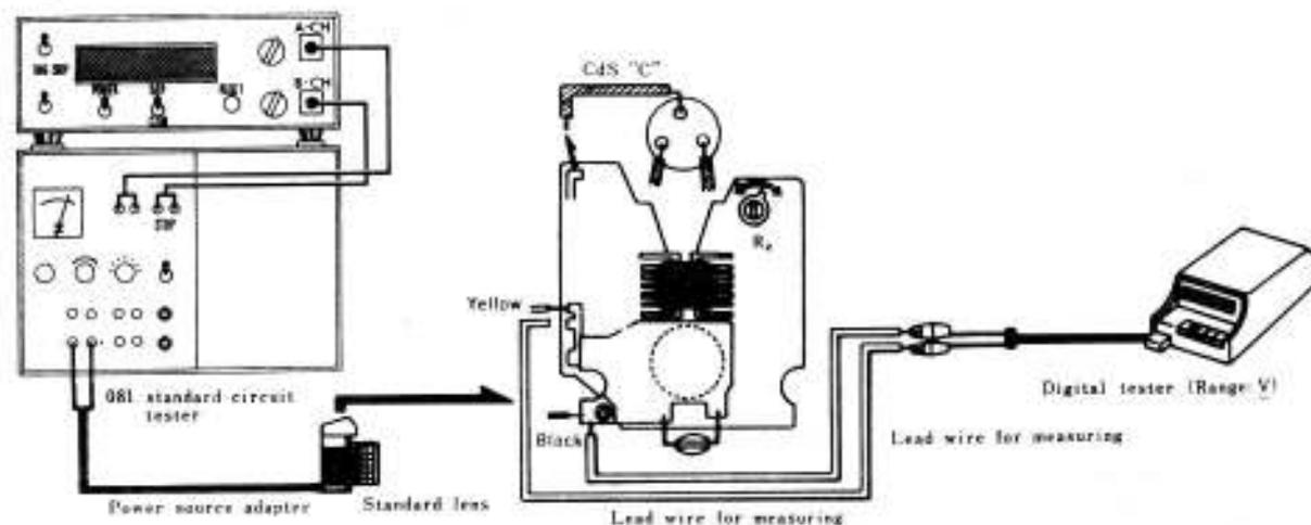
3. With Pv button of the body depressed (Pv SW: ON), measure voltages (mV) for lens F 2.8 and for lens F 16, and make adjustment by means of  $R_2$  so that the difference will be of the value shown in the table below. Voltage decreases if  $R_2$  is turned right and it increases if  $R_2$  is turned left.
