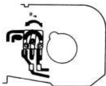
3. After 1/4 adjustment, release the shutter at a speed of 1/1000, make adjustment by means of  $R_{12}$  (resistance for short split-second timing adjustment) so that the measured value may approach the standard (0.98ms).  $R_{12}$  gains speed if turned left and loses speed if turned right. (Refer to the figure below).
