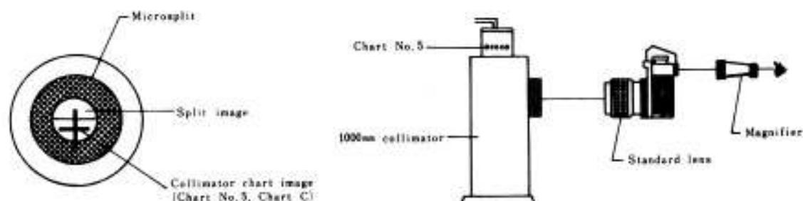
2. In a condition where white lines of the standard lens coincide, loosen 3 set screws of the penta holder (9111 left screws), raise and lower uniformly the focus adjusting nut B (9112) and, at the position where the vertical lines of the chart image coincide, tighten 9111.
