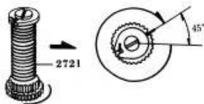
• Using the special tool (Tool No.081-2721-75), turn the gear round in the direction of the arrow mark, and set it at the position shown in the diagram.
