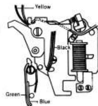
■ **After assembly:** Attach the shutter block to the body, and then attach the shutter base plate (081-0270) and the winding lever (081-0340). (See Page. 13-15 of the disassembly, assembly, and adjustment manual.)
