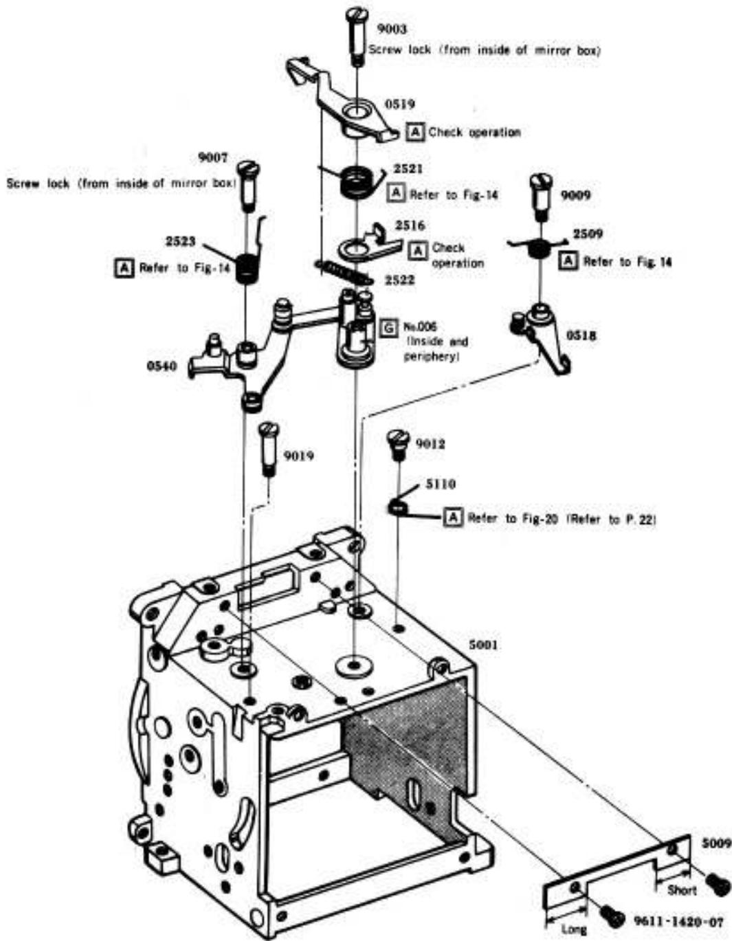
Fig-14 How to engage 2509, 2521, 2523 SP
