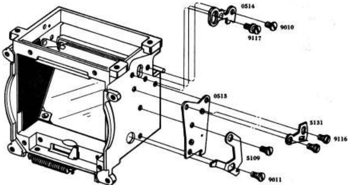
■ After incorporating this, make spacing adjustment of SW. 5.
