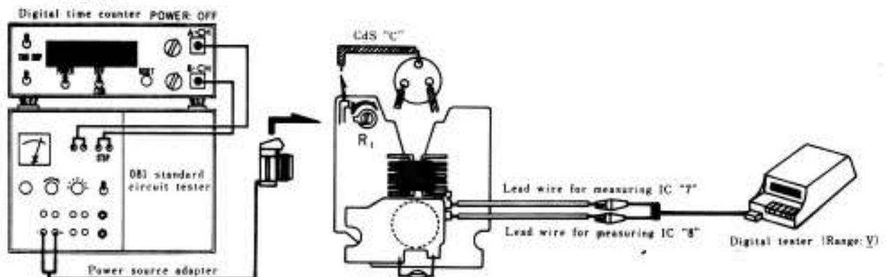
3. Turn  $R_1$  and make adjustment so that voltage (mV) of IC terminals "7" and "8" of the printed base plate A (0432) may be of the value shown in the table below. Voltage decreases if  $R_1$  is turned right and it increases if  $R_1$  is turned left.
