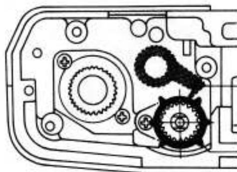
When film advance base plate is attached, set the reversing stop nail A (3048) in the position shown in the figure.
