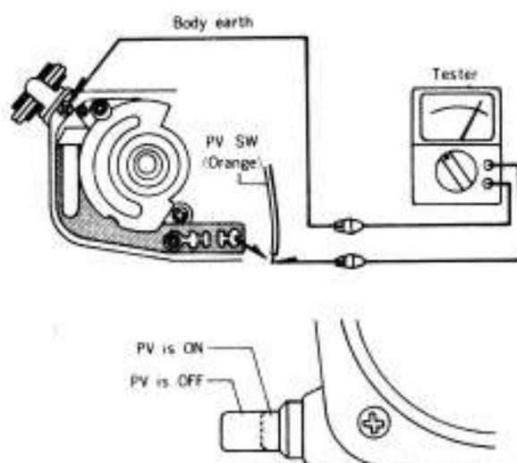
Disconnect the lead wire (orange) of PV SW, connect a tester between the lead wire and body earth, turn the diaphragm button ON and OFF to check if PV SW turns ON and OFF.
