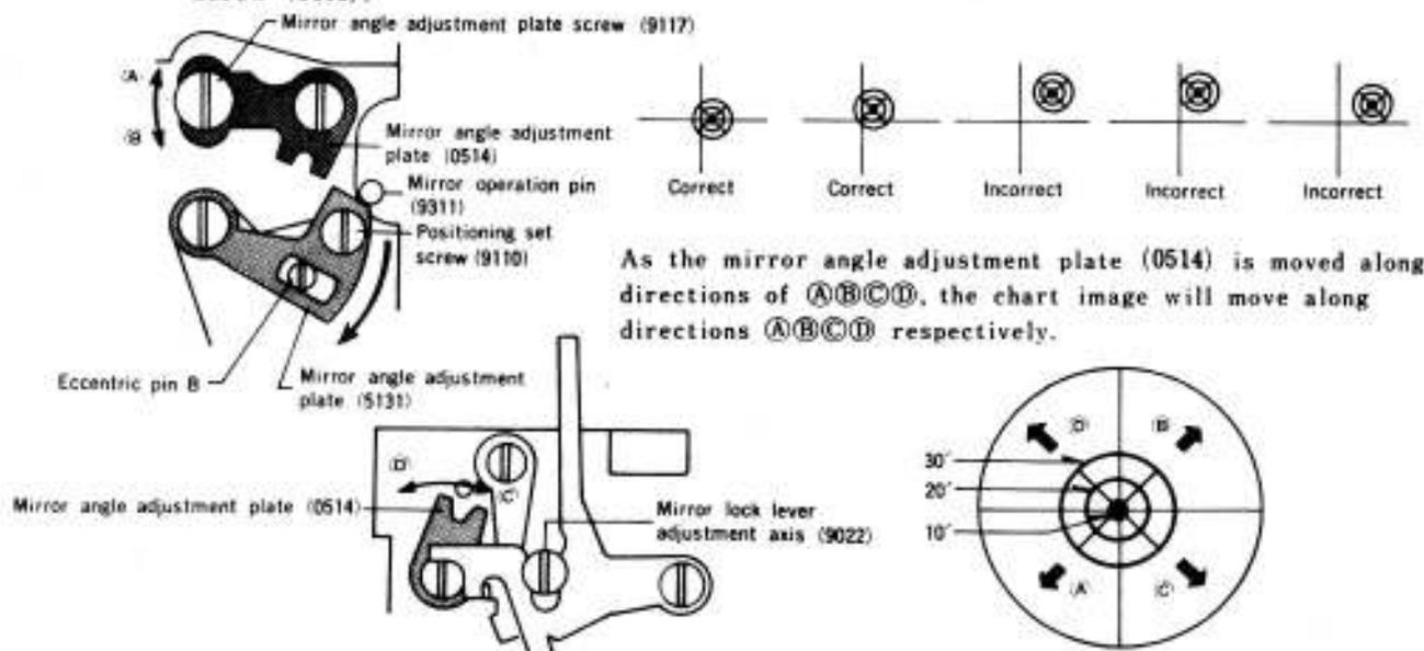
As the mirror angle adjustment plate (0514) is moved along directions of A, B, C, D, the chart image will move along directions A, B, C, D respectively.
