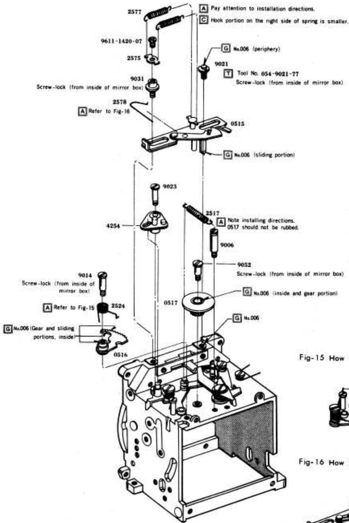
Fig-15 How to engage 2524 SP
