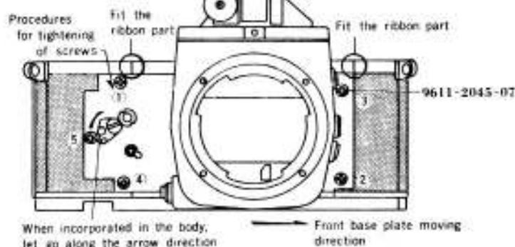
2. After assembling the front base plate, click the shutter at "B" to ensure about ON and OFF of SW 2, SW 3 and SW 4.
