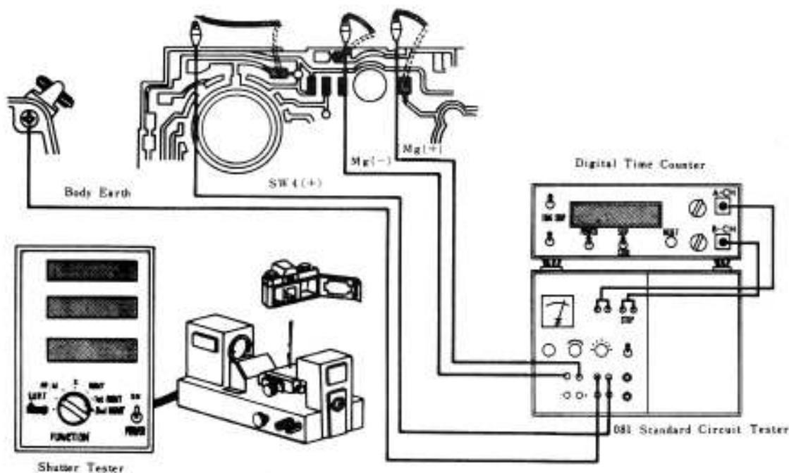
2. Select a shutter speed by the "SS SEL" dial of the 081 standard circuit tester. Press the "RESET" SW of the 081 standard circuit tester, release the shutter, and confirm that the measured figure of 1/1, 1/4 and 1/1000 remains within the range of the rated figures.
