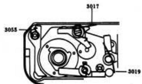
Multiple exposure axis should be positioned after the counter base plate is incorporated.
