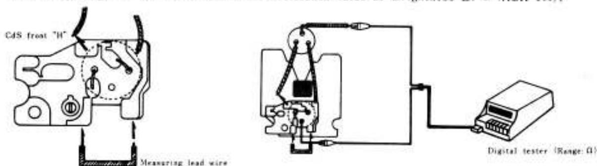
3. Measuring of resistance value of  $R_{LL\ BVS}$  (Resistance value should be within  $16\sim 40K\Omega$ ).
