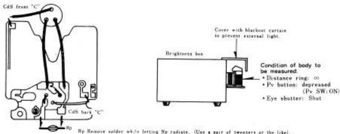
2. Measuring of resistance value of  $R_{LL\ BVS}$  (Resistance value should be within  $88\sim 340K\Omega$ ). Connect between "L"s of CdS (front and back) the measuring wire, remove the solder at "H" terminal of CdS front and connect the digital tester to "C" of CdS (front and back). Set the measuring range at " $\Omega$ " and measure the resistance value at Brightness Ev 5 (ASA 100).
