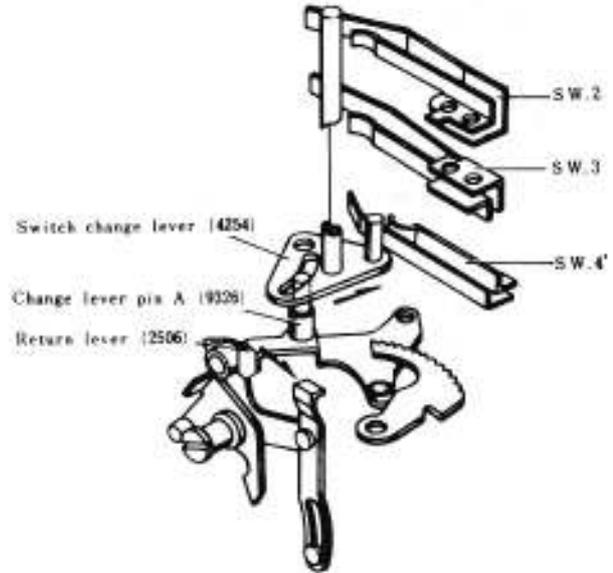
[Diaphragm and On-Off System of PV SW]
