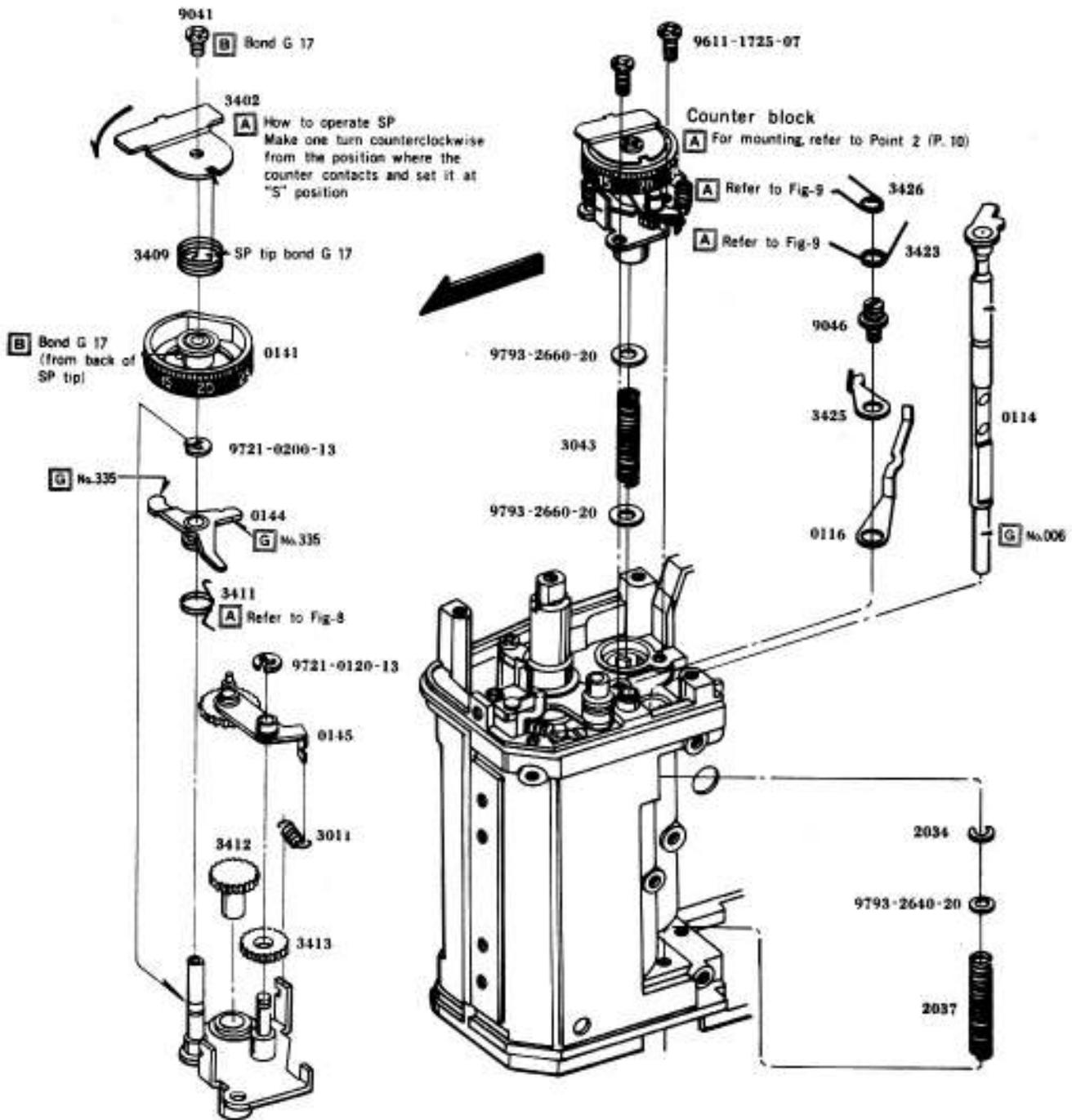
Fig-8 How to engage 3411 SP
