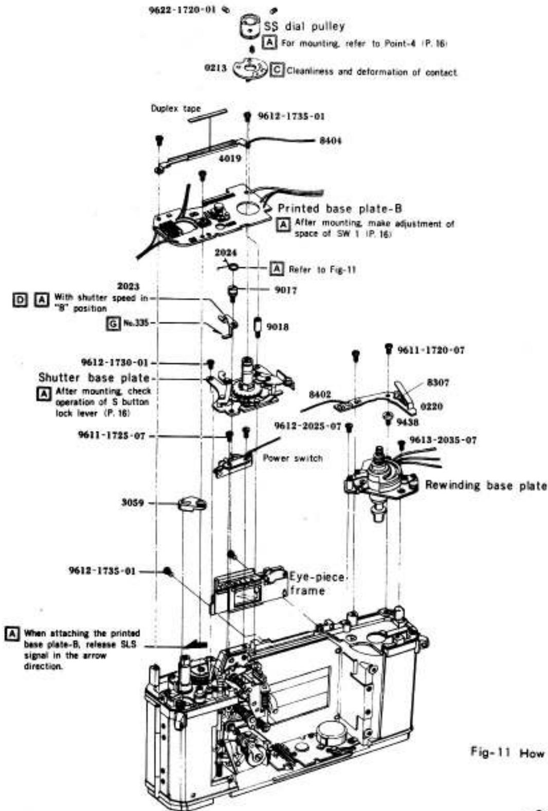
Fig-11 How to engage 2024 SP.
