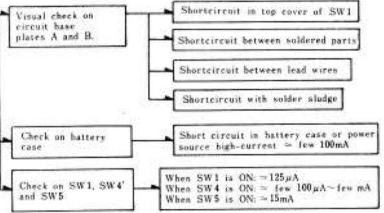
C. Power Sensitivity of Meter (the meter does not indicate the variations equivalent to the varying aperture figure, ASA number, brightness etc.)
