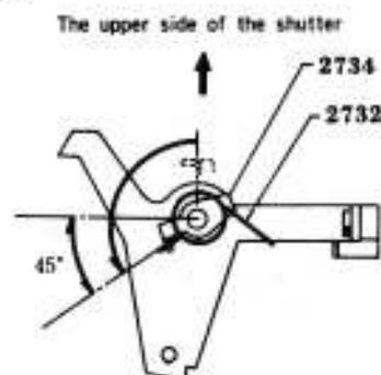
• Turn 2734 round in the direction of the arrow mark, and set it at the position shown in the diagram.
