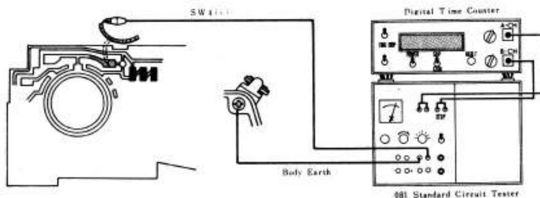
2. Set "S4 SW" of the 081 standard circuit tester to 1/1000 and 1/60, press the "RESET SE" release the shutter, and confirm that the measured figures of 1/1000 and 1/60 remain within the range of the rated figures.
