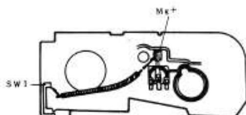
As SW5 is turned ON during shutter release only, short-circuiting it may sometimes be convenient in tracing the causes of trouble. On this occasion, use the lead wire as indicated in the drawing.
