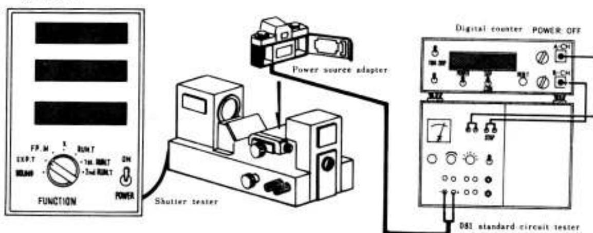
2. Release the shutter at a speed of 1/4, and make adjustment by means of  $R_{10}$  (resistance for long split-second timing adjustment) so that the measured value may approach the standard (250ms).  $R_{10}$  loses speed when turned left and gains speed if turned right. (Refer to the figure below).
